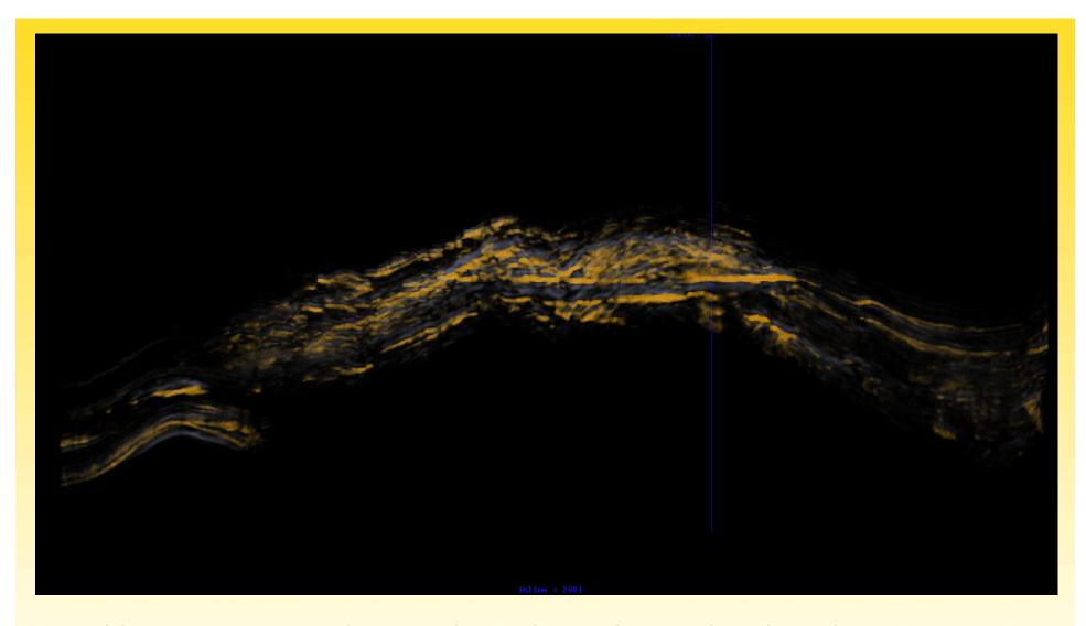
Click image twice to animate - The sequence begins with a view of a structural map showing the various seismic anomalies associated with the Lykos play before zooming in to a close up of the Lykos discovery showing the amplitude response of the gas charged reservoir and ending with a voxel "cloud" display which highlights the flat spot associated with the gas water contact intersected by the well as well as deeper contacts which were not penetrated and represent upside potential.
