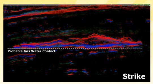
Opacity stacks through Fortuna seismic amplitude volume showing anomalous response of gas reservoirs
