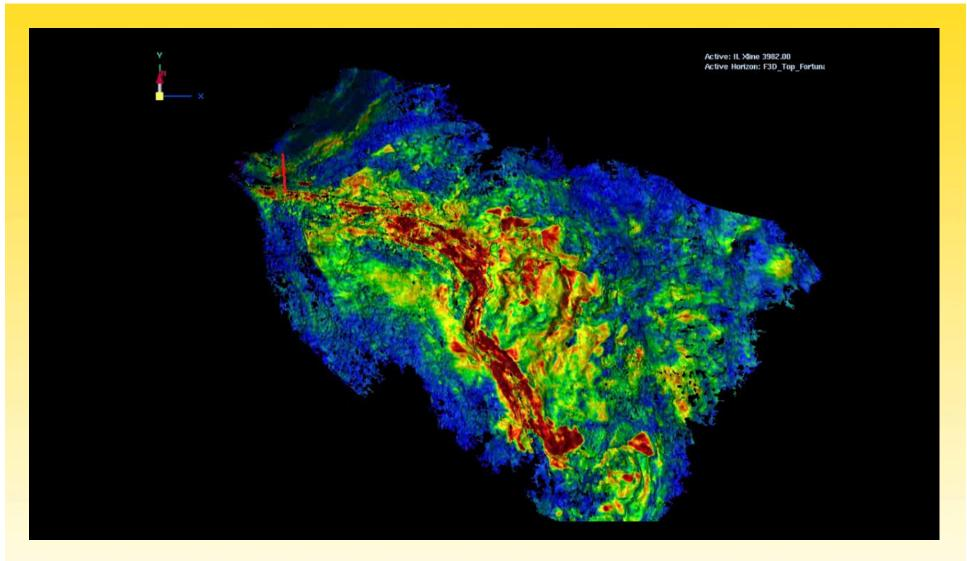
Click image to animate - The sequence begins with a perspective view of a surface through the Fortuna Fan overlaid with seismic amplitudes before progressing through an animation within the seismic volume and ending with a three dimensional voxel or "cloud" display of the reservoir within a far offset time volume which illustrates the clear definition of what is interpreted to be the gas water contact.
